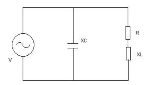
$$V = 230 \cdot sen (wt) V \quad Xc = -10j \Omega \quad XL = 10j \Omega \quad R = 10\Omega$$
